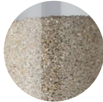
quartz sand makes the glass effect of the glaze
