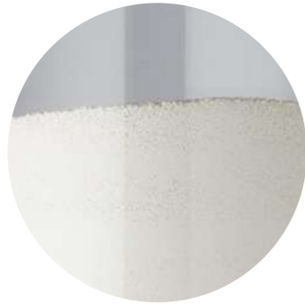
pressing granules he hollow granules are being used for the production of the plates
